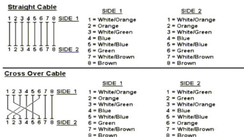
Figure A-1: Straight-Through and Crossover Cable
