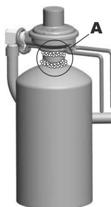
If you cannot stop a leak, remove gas cylinder from regulator and check for damaged threads, dirt and debris on regulator and gas cylinder. Also check to see if anything is obstructing flow of gas at regulator and gas cylinder openings. Remove any obstruction that may be found and repeat leak test. **If threads are damaged on either regulator or gas cylinder, replace.** Order new parts by giving the serial, model number and name of items needed to the Grill Service Center at **1-800-232-3398**.
