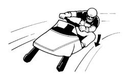
This procedure should be practiced at low speeds many times, in a large flat area with no obstacles. Once you have learned this technique, you should be able to perform it at higher speeds or in tighter curves. Lean more as the turn gets sharper or is made at higher speeds.
