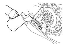
Recommended drive chain oil: SAE 75W or 80W API GL-3 Gear oil
