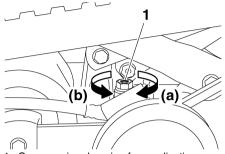
Compression damping force adjusting screw
