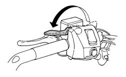
Be sure the engine stop switch is in the run position. The starter motor cannot be operated when the engine stop switch is in the off position.
