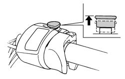
3. Turn the main switch to the start position and release it when the engine starts. NOTICE: Release the switch immediately after the engine starts. If the engine fails to start, release the switch, wait a few seconds, then try again. Each attempt should be as short as possible to preserve the battery. Do not crank the engine more than 10 seconds on any one attempt. [ECS00331]
