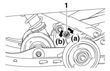
Compression damping force adjusting screw Compression damping force setting: Minimum (soft):
