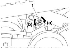
Compression damping force adjusting screw Compression damping force setting (rear):
