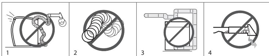
1. Restricting your dryer with a poor exhaust system.
