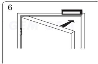
6 Close the door. Measure the correct position by bringing the armature plate close to the contact surface of the electromagnetic lock.
