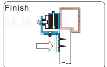
Finish Once the position is correct, use the screws to permanently mount the Z bracket on the door frame. This should be the last step.
