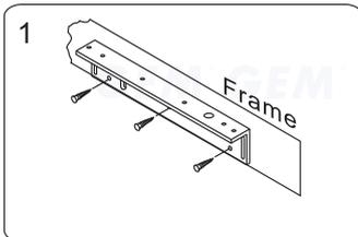
1 Find a mounting location on the door frame for the L bracket. Make sure that the door is still closeable.
