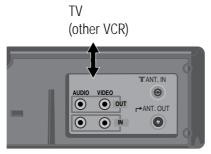
To copy to your video **from another video machine**, connect the two machines with a cable between their A/V sockets and select as programme "AV" using the AV button.
