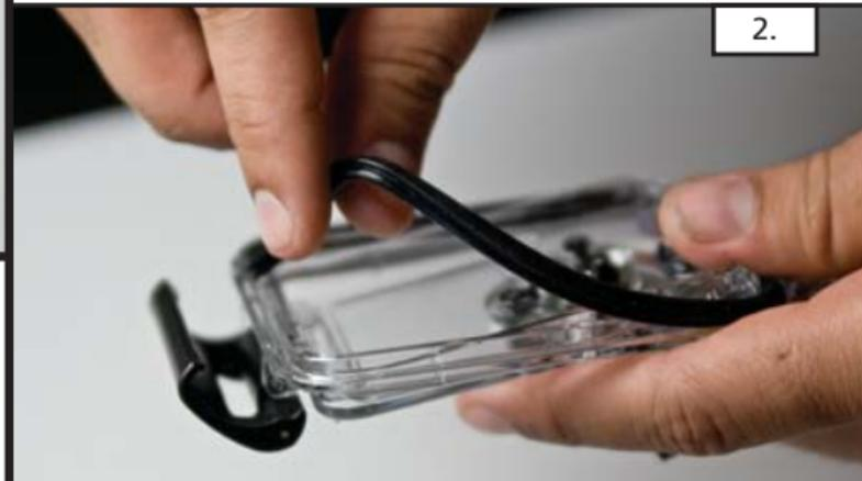
3. To install a new or clean T-Seal, start at any corner, push the T-Seal into the corner and run your finger along the T-Seal pushing it into the Case Contact Surface.
