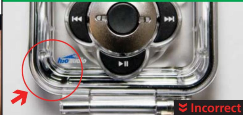
The misaligned T-Seal becomes pinched between the base and lid (as shown) creating an opening in the case that will cause the case to flood.
