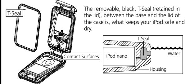
The removable, black, T-Seal (retained in the lid), between the base and the lid of the case is, what keeps your iPod safe and dry.
