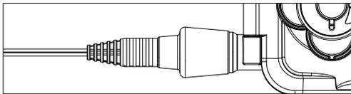
2. Insert the headphones into the stereo jack of the housing, ensuring that the plug mates securely into the SealTight™ Connector.
