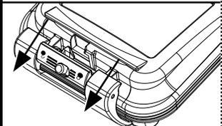
2. While holding the latch button towards the unlock icon, push away from the case to open the latch.
