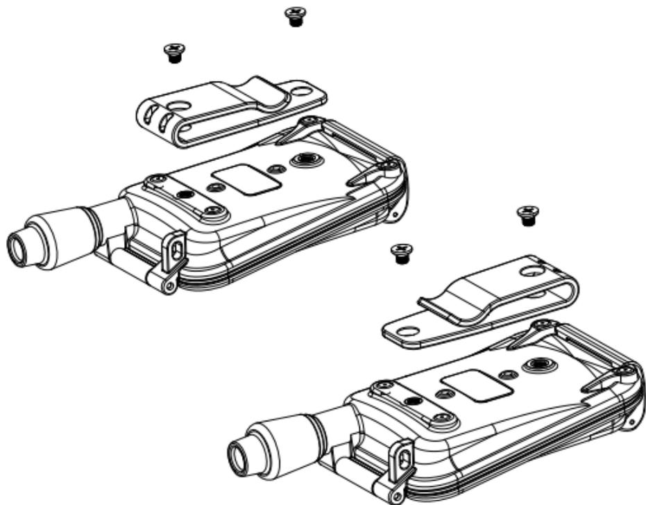
The Belt Clip can be reversed to change the access direction of the stereo jack.
