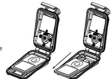
NOTE: Do not disturb the T-Seal during removal of the player. If the T-Seal is moved, Please use the case lid to completely seat the T-Seal.
