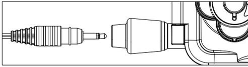
1. To create a waterproof connection, align the 3.5mm stereo plug on the headphones with the stereo jack of the case.
