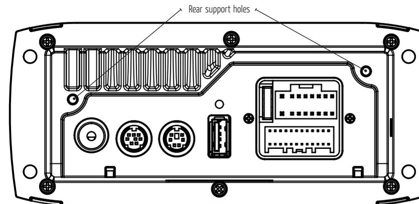
In some cases a rear support strap (not supplied) may be required. Please use the two holes indicated above, to attach the strap using two 8 gauge x 8mm self-tapping screws (not supplied).
