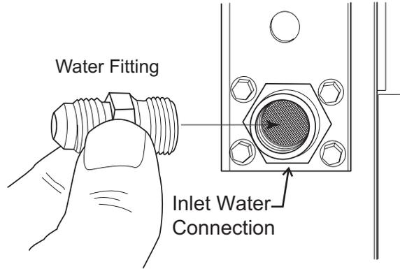
Water cooled models have the same inlet fitting plus an additional 3/8" FPT condenser inlet water connection.
