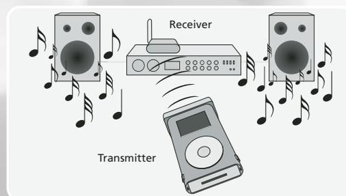
The iParty creates a wireless connection between your iPod and your audio system. Just click your iPod onto the iParty transmitter. The receiver can be connected to your hifi system via the RCA cable included. The transmitter has its own rechargeable battery and does not use any power from your iPod. A second rechargeable battery is included and can be charged up in the receiver. This means you always have a fully charged battery available.
