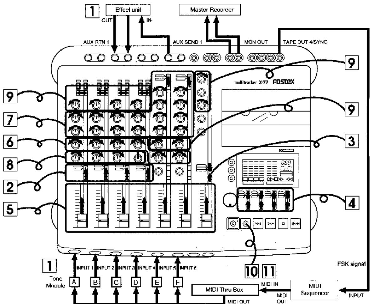
**1 Connections between the X-77 and master recorder and effect unit**
