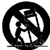
A appliance and cart combination should be moved with care. Quick stops, excessive force, and uneven surfaces may cause the appliance and cart combination to overturn.
