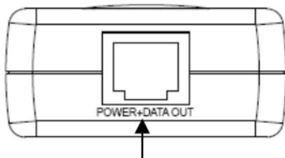
**POWER+DATA OUT:** Connect to the PD or PoE Splitter with a CAT5 UTP cable.
