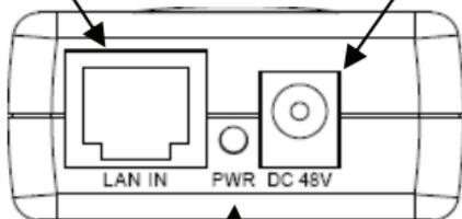
**PWR:** Power LED, a steady green light indicates that the PoE system has detected the PD or PoE Splitter and the power adapter is working properly.
