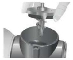
7. Once the burr-shaft assembly is in the motor housing, rotate the assembly until it falls into place.
