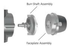
4. Using the burr-cleaning brush, clean the burr mounted on the burr-shaft assembly and the burr mounted within the motor housing.
