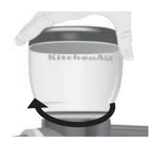
Slide the coffee bin onto the bin platform; the bin seal plate on the motor housing will compress slightly to accommodate the bin. Make certain the bin is centered in the middle of the bin platform.
