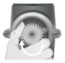
6. When the burrs are touching, turn the grind control gear counter-clockwise 1 "click" or detent. The grating or "rubbing" sound will stop. Turn off the mill by flipping the On/Off Switch to the "Off" position. The mill is now calibrated to provide maximum fineness.
