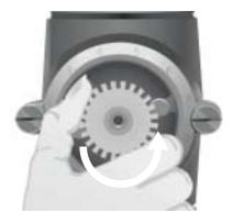
4. Re-attach the grind control dial, making certain the dial indicator points to level "1".
