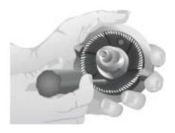
3. Remove the burr from the motor housing by turning the two burr-mounting screws counter-clockwise until free.
