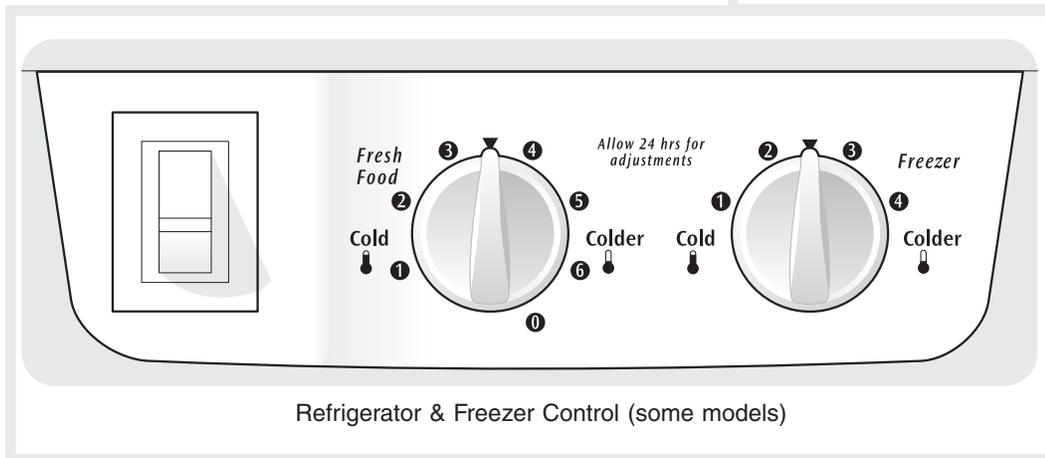
**\* IMPORTANT:** Turning the refrigerator temperature control to “0” turns off the compressor, but does not disconnect the power to the light bulb and other electrical components. To turn off power to your refrigerator, you must unplug the power cord from the wall outlet.
