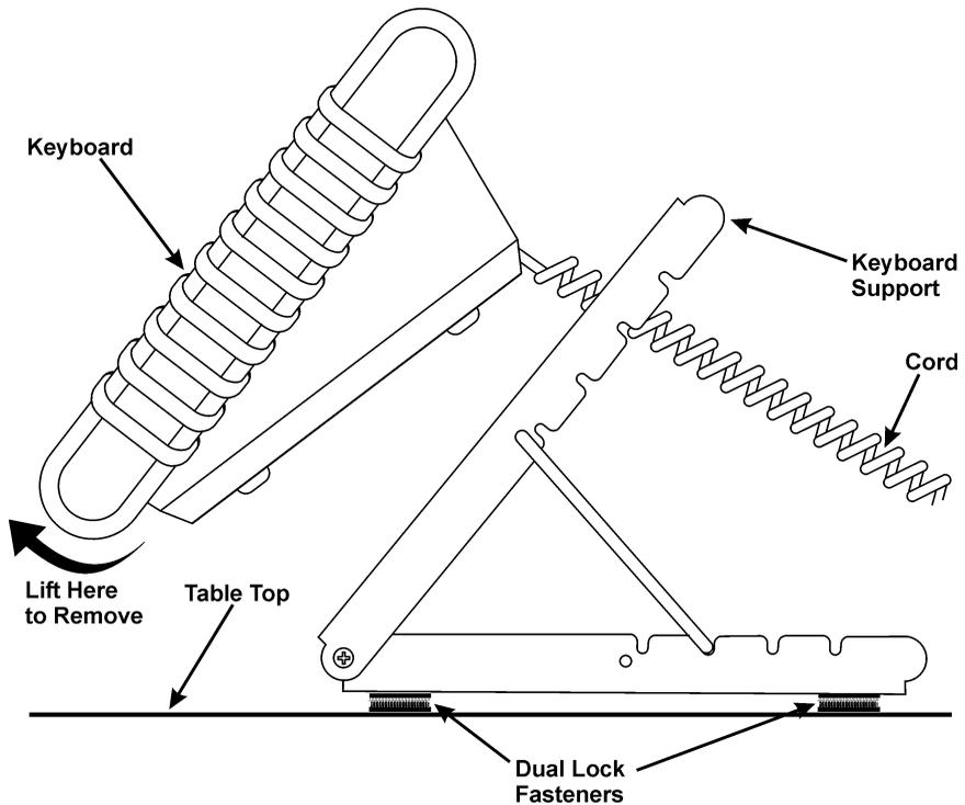
To remove the keyboard from the stand, lift the keyboard from the bottom.
