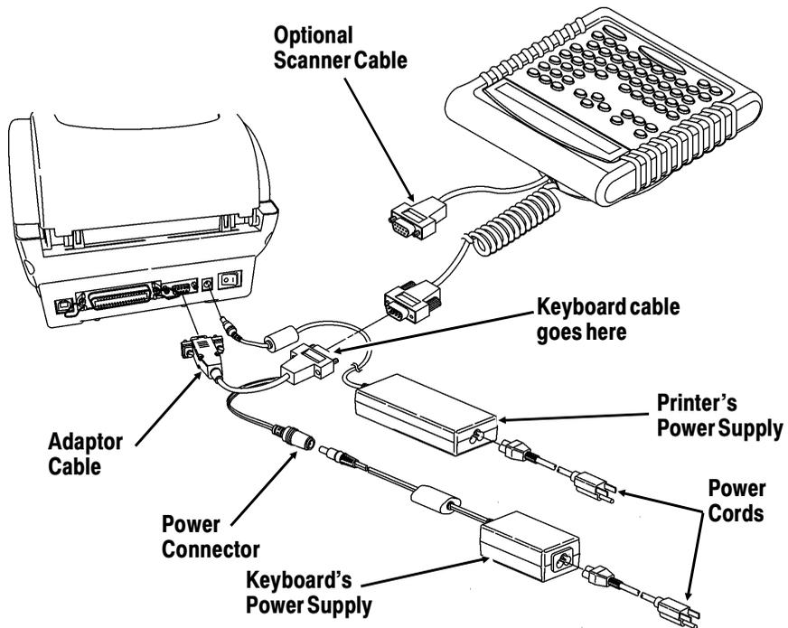
3. Secure the other end of the adaptor cable to the 9-pin port on the printer. Tighten the screws on the cables.
