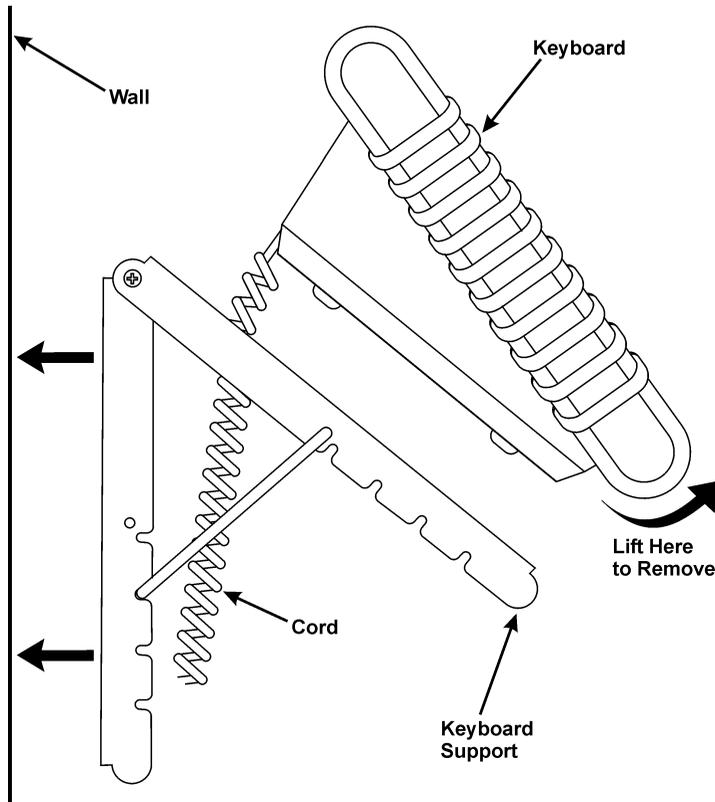
To remove the keyboard from the stand, lift the keyboard from the bottom.
