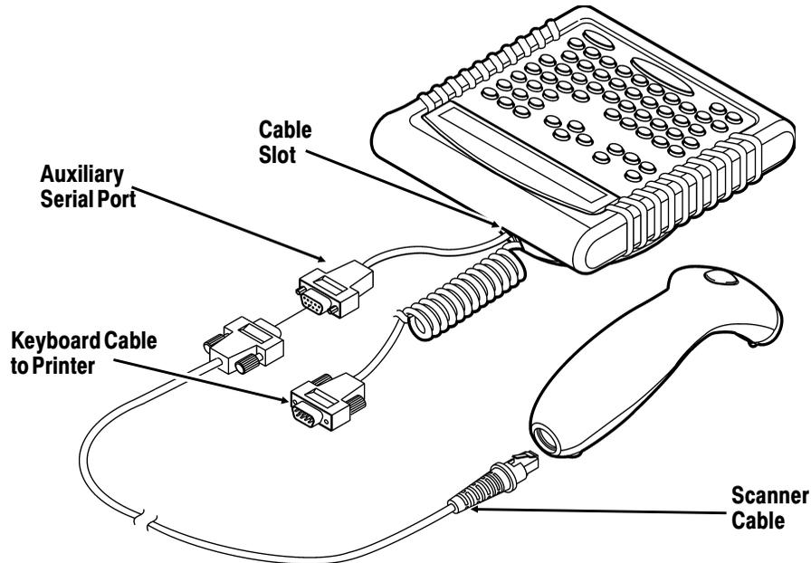
4. On the scanner, connect the RJ45 male connector end of the cable into the scanner. You will hear it click into place.
