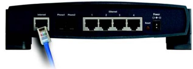
Figure 4-6: Connect the Broadband Modem
