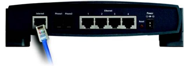
Figure 4-1: Connect the Broadband Modem
