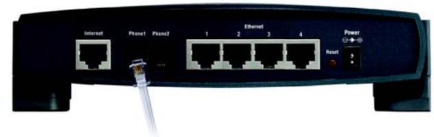
Figure 4-7: Connect a Telephone
