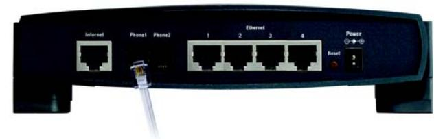
Figure 4-2: Connect a Telephone
