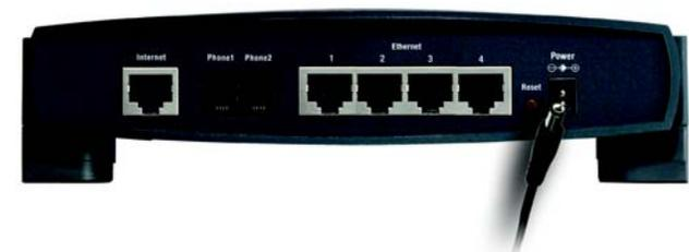
Figure 4-4: Connect the Power
