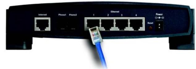
Figure 4-8: Connect the Other Router
