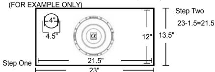
The wood that we are using is 0.75" thick
