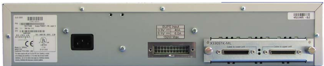
Figure 6.5 P334T-ML DC Back Panel (without Stacking Sub-module installed, BUPS-ML connector cover plate shown)
