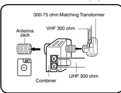
Connect the UHF 300 ohm twin-lead wire to the Combiner (not supplied). Connect the VHF 300 ohm twin-lead wire to the 300-75 ohm Matching Transformer. Attach the Transformer to the Combiner, then attach the Combiner to the Antenna Jack.
