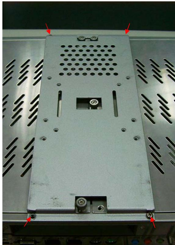
2. Fix the Wall mount bracket kit in back of the VESA bracket kit by 4 screws.
