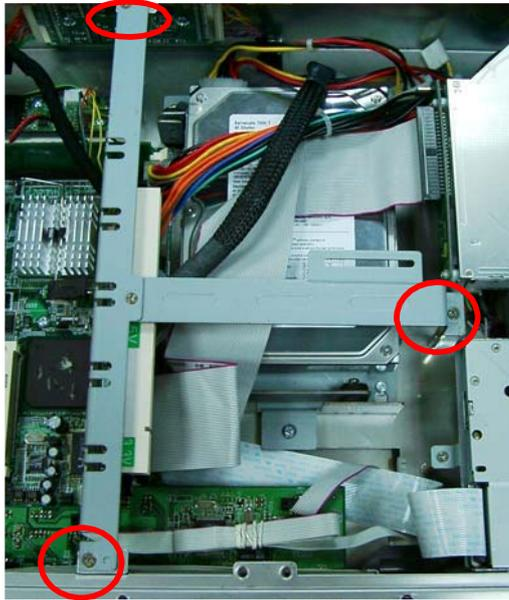
3. Secure 2 screws to fix the CD-ROM PCB board.
