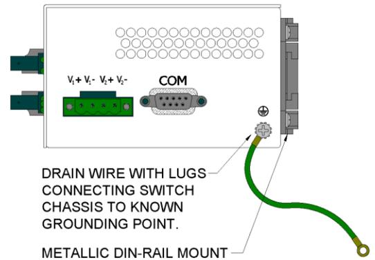
Note: Before applying power to the grounded switch, you must use a volt meter to verify there is no voltage difference between the power supply's negative output terminal and the device chassis grounding point.
