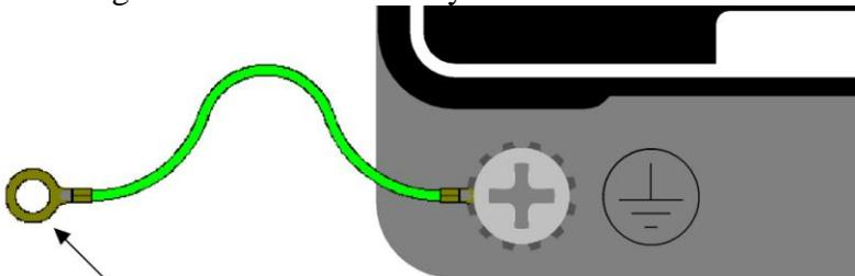
Drain wire with lug connecting switch chassis to known grounding point.
