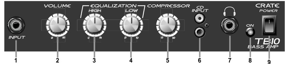
1. **INPUT:** Connect your bass here by means of a shielded instrument cable.
