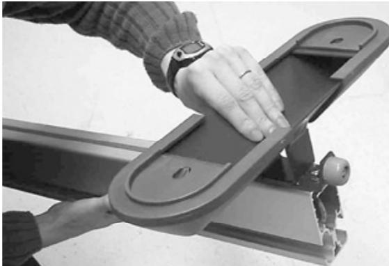
**NOTE!** When fitting the leg to the rear end of the rail, make sure that the rubber seat stopper is at the front!
