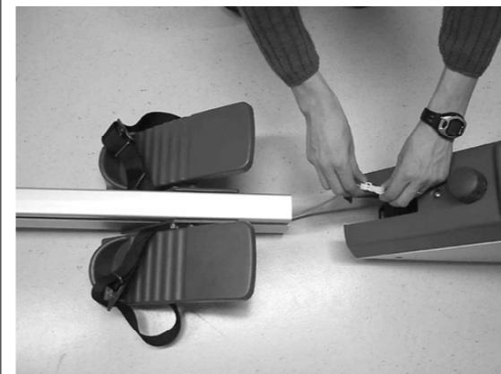
Push the rail into place on the frame so that the thin metal strip on the frame fits into the groove in the rail bottom. Push the rail until it reaches the stopper at the end of the strip.
