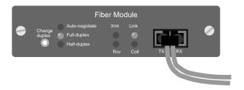
This is a Fiber Module plugged into a hub running at either 10 or 100 Mbps. The module is then connected to an Intel Express 10/100 Fast Ethernet Switch at full-duplex using 62.5/125-micron fiber optic cable. The module was forced to full-duplex to ensure a connection to the switch. The maximum cable distances are shown below.
