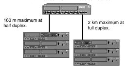
Intel Express 10/100 Stackable Hubs. Each stack has a Fiber Module installed.
