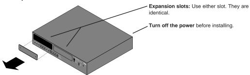
2. Plug either the Ethernet Module or the Fiber Module into a slot, using the retaining screws to secure the module to the hub.
