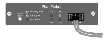
This is a Fiber Module plugged into a hub running at either 10 or 100 Mbps. The module is then connected to another Fiber Module using 62.5/125-micron fiber optic cable. Both modules auto-negotiated to full-duplex by default.
