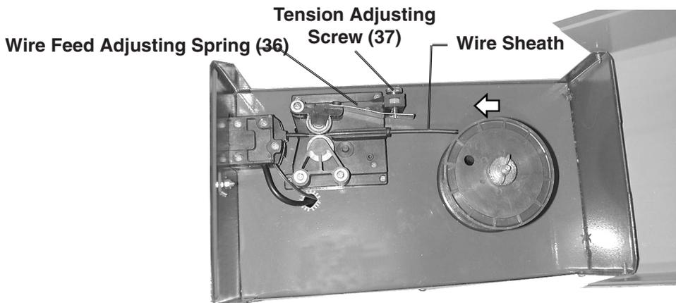
1. Press on the Cover Locking Spring (8), then lift the Cover (31) using Handle (30) to expose the Wire Feed Unit (23).
