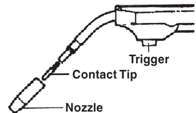
10. Turn the Contact Tip counterclockwise and remove.
