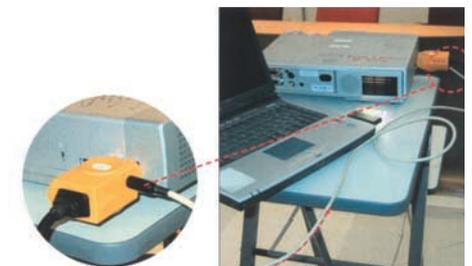
The USB loop is connected with the safety cord SK300 and USB interface of an external unit. If the USB plug is disconnected, the pre-activated 100 dB will go off.
