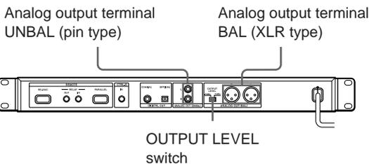
**When BALANCE output (XLR type) terminal is used, output level can be changed by OUTPUT LEVEL switch.**
