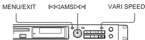
**1** During playback or in pause mode, press the VARI SPEED button. "VARI SPEED" indicator lights up.
