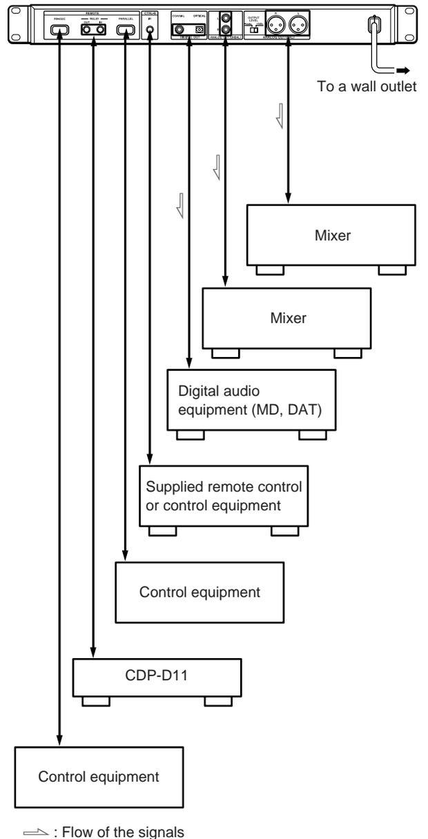
**To use the supplied remote control as the wired remote control**
