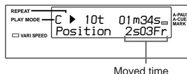
The point can be moved up to 8 seconds forward or backward in 5 frames interval (5 frames = approximately 0.0667 seconds).
