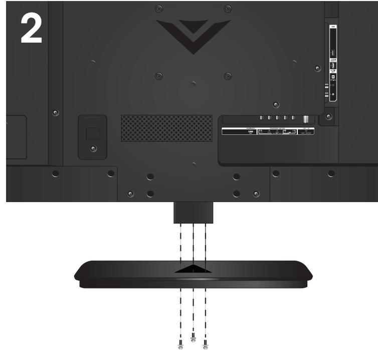
Align the base with the neck and tighten the three (3) included M4 10mm Phillips screws using a Phillips screwdriver as shown.
