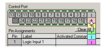
Now, place the cursor in the ACTIVATED COMMAND column for Logic Input 1 and select INSERT, MACRO, 0 ("MUTE ON"). Now, whenever the switch goes Active Low (0V DC), the Vortex Device will execute Macro 0.
