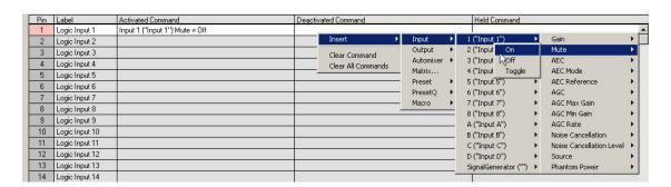
Now, right click in the Held Command column for Logic Input 1 and select Insert, Input, 1, Mute, Off. Now, whenever the switch goes Active Low (OV DC), the Vortex Device will unmute Input 1.
