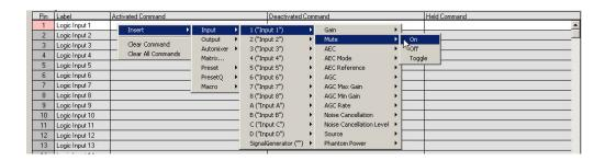
Now, right click in the DEACTIVATED COMMAND column for Logic Input 1 and select INSERT, INPUT, 1, MUTE, OFF. Now, whenever the switch goes Active High (+ 5V DC), the Vortex Device will unmute Input 1.
