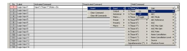
Do not assign any command to the Held Command column.
