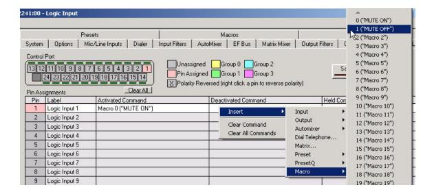
Now, right click in the Held Command column for Logic Input 1 and select Insert, Macro, 0 "(MUTE ON"). Now, as long as the switch is held down, the Vortex Device will execute Macro 0.
