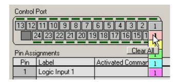
Now, right click in the ACTIVATED COMMAND column for Logic Input 1 and select INSERT, INPUT, 1, MUTE, OFF. Now, whenever the switch goes Active Low (OV DC), the Vortex Device will unmute Input 1.
