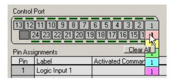
Now, right click in the ACTIVATED COMMAND column for Logic Input 1 and select INSERT, INPUT, 1, MUTE, ON. Now, whenever the switch goes Active Low (0V DC), the Vortex Device will mute Input 1.
