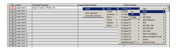
Now, right click in the Held Command column for Logic Input 1 and select Insert, Input, 1, Mute, On. Now, as long as the switch is Active Low (OV DC), the Vortex Device will mute Input 1.
