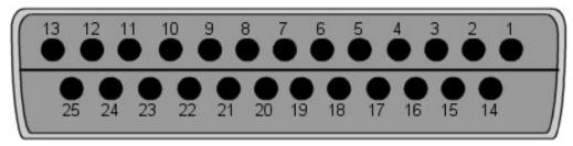
The Logic Output port is a female DB-25 connector where pins 1-20 can be programmed. Pins 21-25 are ground pins. Each pin can source up to 20 mA of current and each ground pin can sink up to 100 mA of current.
