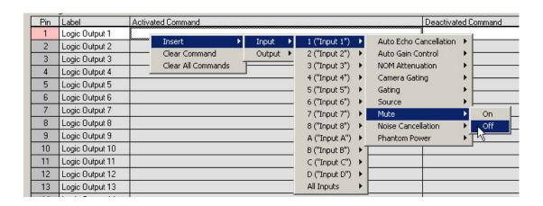
Next, right click in the DEACTIVATED COMMAND column for Logic Input 1 and select INSERT, INPUT, 1, MUTE, ON. Now, whenever the microphone is muted (Mute = True), the LED will not illuminate on the MX392.
