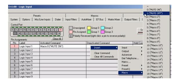
Do not assign any command to the Held Command column.
