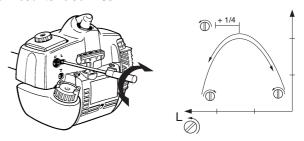
CAUTION! If the cutting attachment rotates when the engine is idling the idle adjustment screw T should be turned anticlockwise until the cutting attachment stops.
