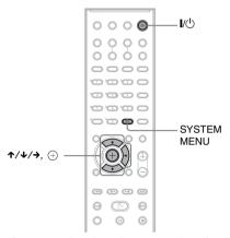
After connecting the AC power cord (mains lead), the demonstration appears in the front panel display. When you press \( \bar{\ll} \subset \) on the remote, the demonstration turns off.
