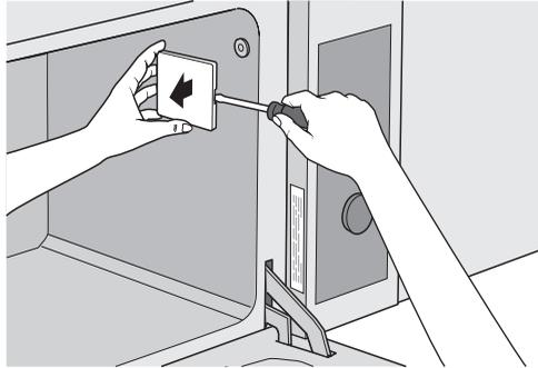
3. Replace oven halogen light bulb (25 W, 12 V, heat-resistant up to 300 °C).
