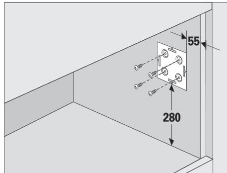
2. Fix the clips to both side walls on the appliance.
