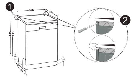
*Warning:*The stand part which will settle the machine under it by removing its worktop has to be stable in such a way not to allow balance disorder.
