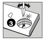
To put rinse aid, remove the rinse aid compartment cap by turning it.
