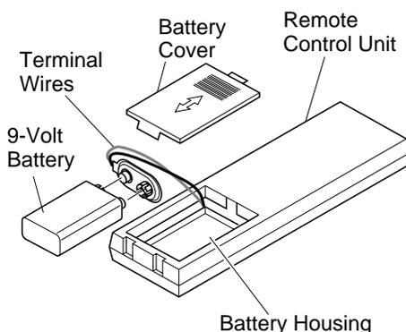
**Figure 48 - Installing Battery in Hand-Held Remote Control Unit**
