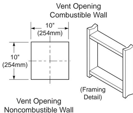
**Figure 22 - Vent Opening Requirements**
