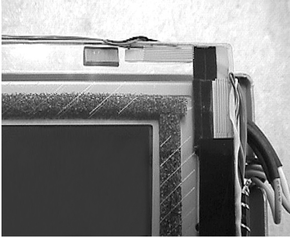
Figure 2.9 Attaching double-sided adhesive tape to the touchscreen
