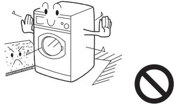
10. Keep away from heat sources and direct sunlight to prevent plastic and rubber components from aging.
