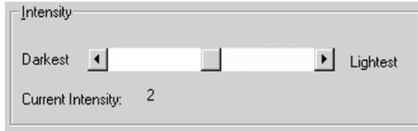
The Intensity control offers five settings, from darkest to lightest. Slide the control toward Darkest to make the image darker on film, or toward Lightest to make the image lighter on film. (Some film packs may require an adjustment to compensate for a slight speed variation.) Leave it at the center setting, 2, unless needed.
