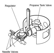
NOTE: POL fittings are made with a metal to metal seal and must be made very tight to prevent leaking. Make sure to not cross-thread fittings while tightening.
