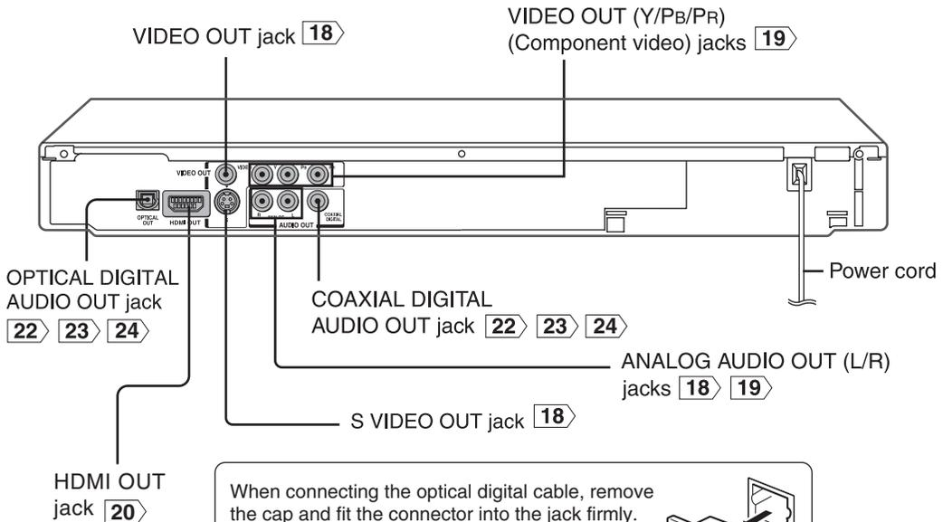
When connecting the optical digital cable, remove the cap and fit the connector into the jack firmly. When not using the jack, keep the cap inserted to protect it from dust intrusion.
