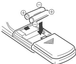
Make sure to match the + and – on the batteries to the marks inside the battery compartment.
