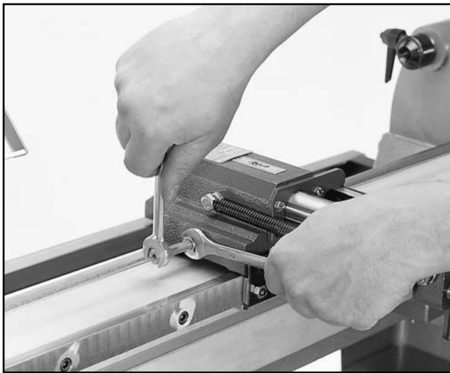
Figure 8. Adjusting carriage cable tension.
