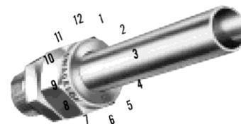
3. Hold the fitting body steady with a backup wrench and tighten this nut  $1\frac{1}{4}$  turns. Watch the scribe mark, making one complete revolution and continue to the 9 o'clock position.
