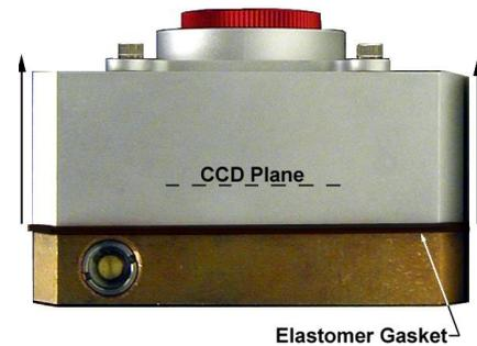
10. Remove the elastomer gasket.
