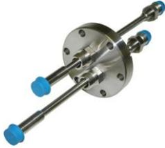
**Vacuum Compatible Camera Flanges:** The  $2\frac{3}{4}$ " ConFlat flange with two pipes ( $\frac{1}{4}$ " OD) and VCR fittings (2825-0562) (or with Swagelok fittings (2825-0447) for earlier systems) and the  $4\frac{1}{2}$ " ConFlat flange with 25-pin D-sub connector (2825-0448) are included with the system.
