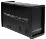
**Electronics:** The ST-133 controller is a compact, high performance CCD Detector Controller for operation with Princeton Instruments brand\* detectors. Designed for high speed and high performance image acquisition, the ST-133 offers data transfer at speeds up to 1 megapixel per second, standard video output for focusing and alignment. A variety of A/D converters are available to meet different speed and resolution requirements.
