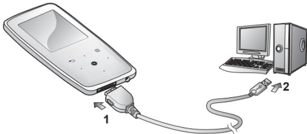
1. Connect the larger end of the USB cable to the USB Connection Port on the bottom of the player.
