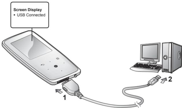
1. Connect the larger end of the USB cable to the USB Connection Port on the bottom of the player.
