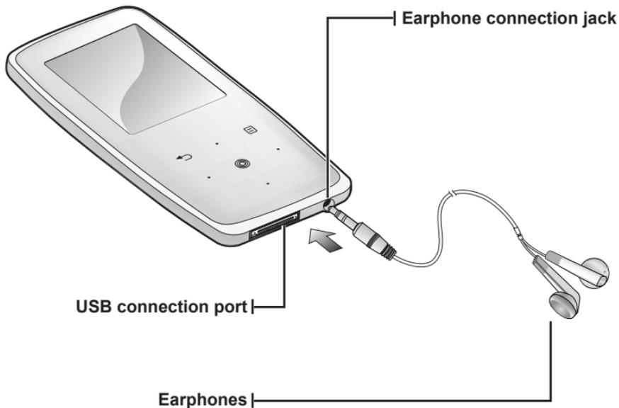
Labeled “L” for the left earpiece and “R” for the right earpiece. Also serves as an antenna for FM Radio in the MP3 player. Disconnecting the earphones during music or video playback will pause the playback.
