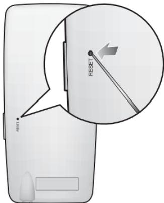
Press the Reset hole at the rear of the player with a pointed object such as a safety clip.
