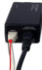
3. Connect a CAT-5 cable from a switch to the TPE-111GI's DATA IN port.
