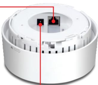
2. Connect the RJ-45 cable from the Switch/Hub to the **LAN** port on the Access Point.
