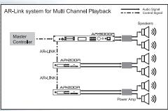
Using the AR-Link function users can build a 64-track simultaneous playback system. One AR-3000R master device can lock up to 31 units of AR-3000R or AR-200R together for sample accurate playback.
