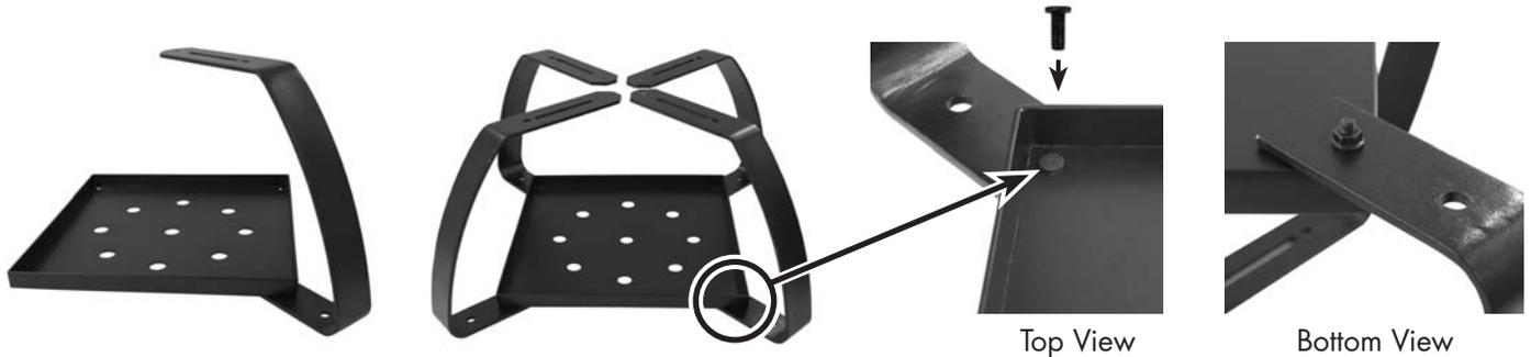
2. Align Grill Support Base on Cart Legs. Insert 4 Carriage Bolts into **center holes** on Grill Support Base connecting it to Cart Legs with Nuts. **LOOSELY TIGHTEN** at this stage.
