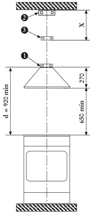
4. Draw a horizontal line through the vertical line at **X**. **X** is a distance between the centre of the top and bottom fixing holes on the upper chimney stack. Mark the centre positions for the **middle bracket** fixing screws (3) at 95mm either of the vertical line (screws not supplied).
