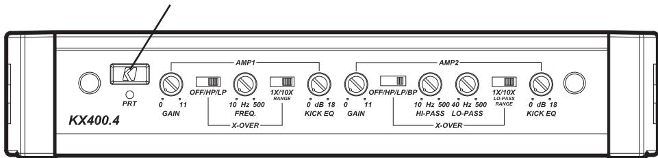
**Automatic Turn-On Selection:** The KX series offers three different automatic turn-on modes that can be selected on the end panel; +12V, DC Offset, and Audio. Using either the DC Offset or Audio mode causes the REM terminal to have +12V out for turning on additional amplifiers.
