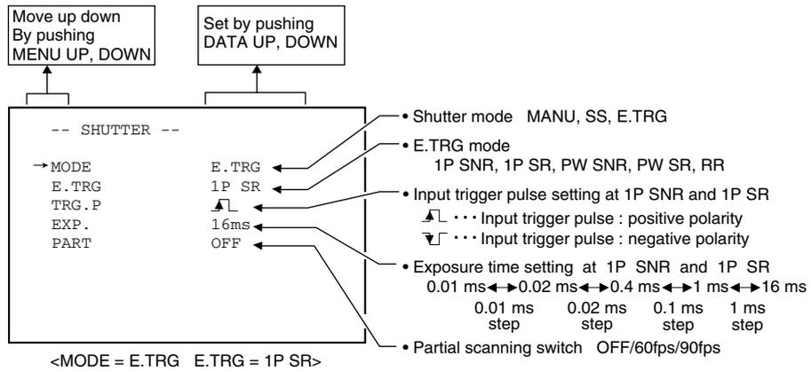
**(a) Changing the polarity of inputting trigger pulse setting**
