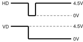
The amplitude level is the representative value when terminated with 10kΩ.
