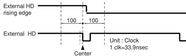
The phase relationship of the external HD and VD should correspond to the center phase (i.e., the external HD falling edge) as illustrated in the above diagram.
