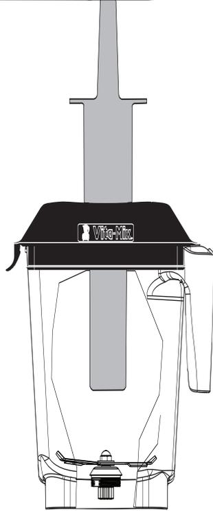
**\*NOTE:** Accelerator Tools have a small step on them. The step prevents the Accelerator Tool from coming into contact with the blades in Vita-Mix polycarbonate containers. Accelerator Tool cannot be used with a one piece non-latching lid.
