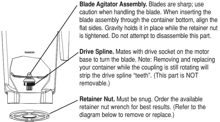
**Blade Agitator Assembly.** Blades are sharp; use caution when handling the blade. When inserting the blade assembly through the container bottom, align the flat sides. Gravity holds it in place while the retainer nut is tightened. Do not attempt to disassemble this part.
