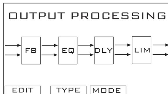
By default, the stereo output menu appears when the Output Processing button (44B) is pressed. If you prefer to work in dual-mono-output or subwoofer mode, return to the main output processing screen by pressing the “mode” soft knob choice.
